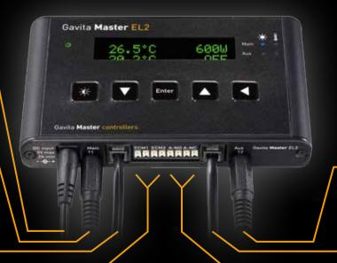
Cage clamp connectors for External Contactor Modules. Safe low voltage connections. Cage clamp connectors for alarm contacts: both normally open and normally closed.
