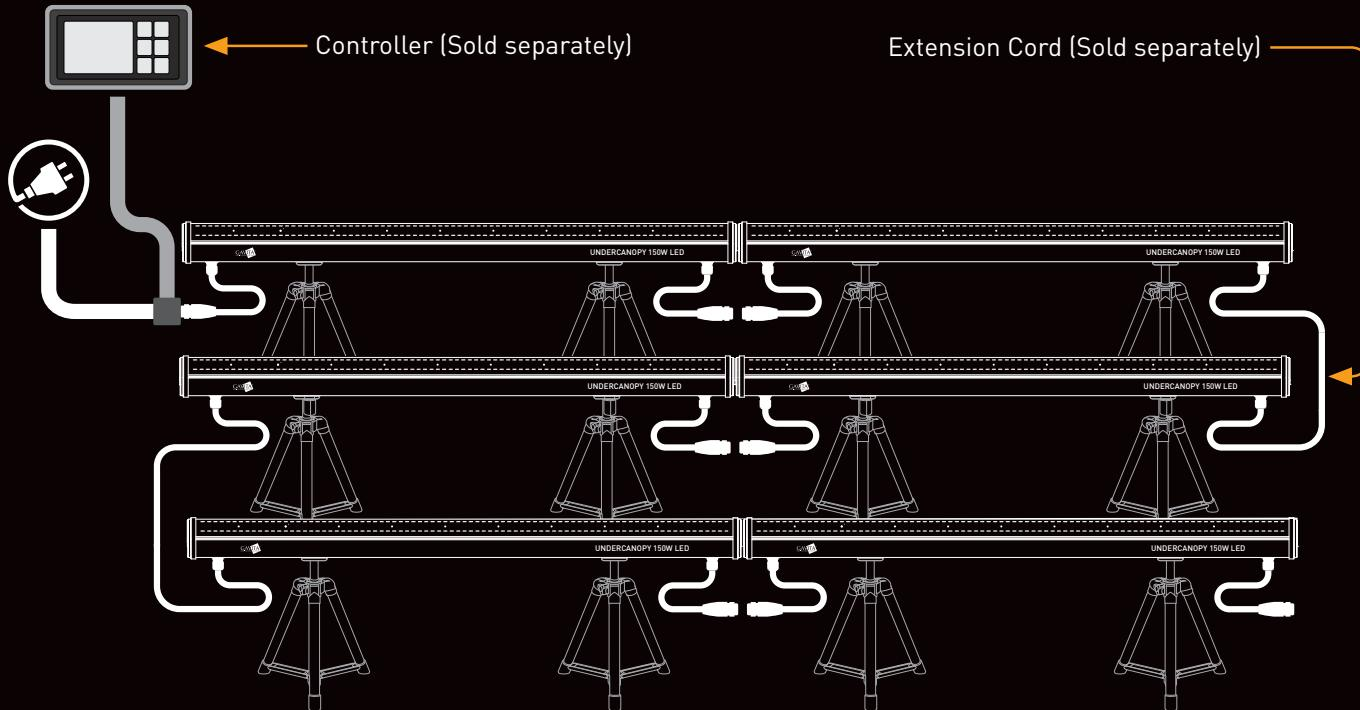
They can be integrated into your existing control systems, with a 0-10V analog control signal, to manage on/off schedules and dimming, either in sync with your top lights or independently. For detailed instructions on mounting, electrical connections, control system integration, and cleaning procedures, please visit the dedicated product pages on our website. There, you'll find comprehensive guides and diagrams to ensure your fixtures are set up and operating correctly.
